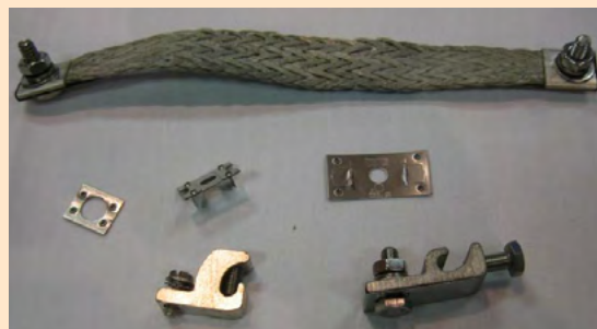
Figure 81. Special bonding jumpers, stainless-steel bonding washers and lay-in lugs may be used to electrically connect separate components or attach equipment grounding conductors.
