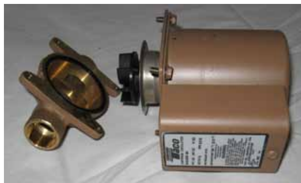
Figure 10-27 – A bronze pump suitable for potable water with the volute separated from the motor. The capacitor is contained in the metal box with the label.
