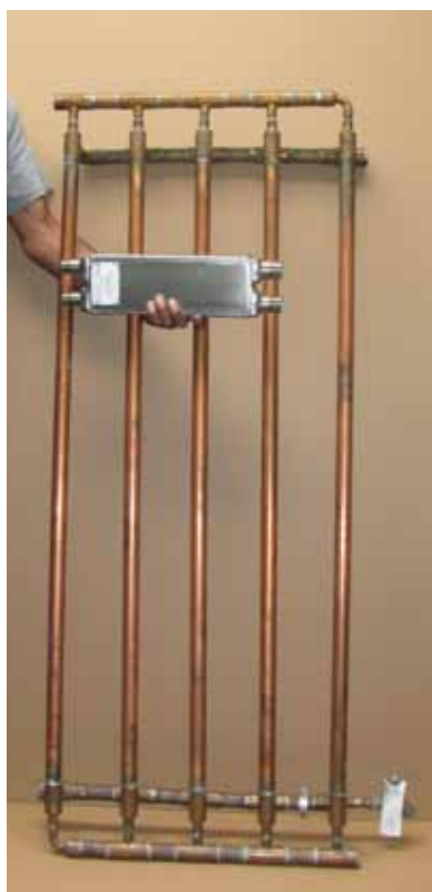
Figure 10-25 — A copper heat exchanger and a stainless flat plate heat exchanger. The tube in the tube exchanger couldn't heat the indoor pool and was replaced with the smaller plate heat exchanger. The plate exchanger was more effective and heated the pool year-round with the same eight collectors due to the increased exchanger surface area and much higher surface-to-volume ratio.
