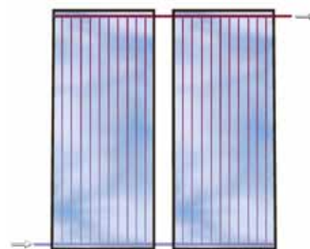
Figure 8-21 — Harp-style flat plate collectors plumbed in parallel. (Courtesy of AET)
