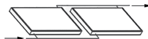
Figure 8-23 — Plumbing harp-style flat plate collectors in parallel when oriented landscape requires extra external piping. (Courtesy of NYSERDA)
