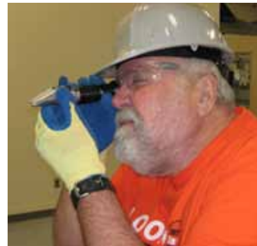
Figure 8-52 — Checking propylene glycol concentration using a refractometer.
