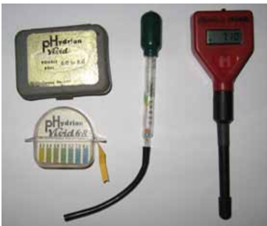
Figure 10-6 - Glycol test equipment — Litmus litmus paper, propylene glycol freeze tolerance tester, and pH meter.
