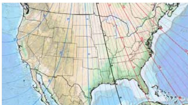
Figure 3-9 — 2010 Isogonic Map of the United States. The dark line in the middle represents the locations where magnetic north and true north are equivalent. Locations east of the line have a western declination; locations west of the line have an eastern declination. For example, the magnetic declination in San Francisco, CA is between 14^{\circ} and 15^{\circ} east. This means that magnetic north is roughly 14.5^{\circ} east of true north there. At the 10^{\circ} blue line, the azimuth angle is 170^{\circ} on the compass. At the 10^{\circ} red line the azimuth angle is 190^{\circ} on the compass. (Courtesy of NOAA)
