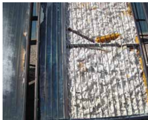
Figure 10-13 – Failure to promptly repair broken glass can cause absorber damage from the wind.
