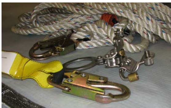
Figure 8-2 — Contents of a roof fall protection kit, including a lanyard, rope grab, and safety rope; a safety harness and a ridge anchor are typically included and not shown.
