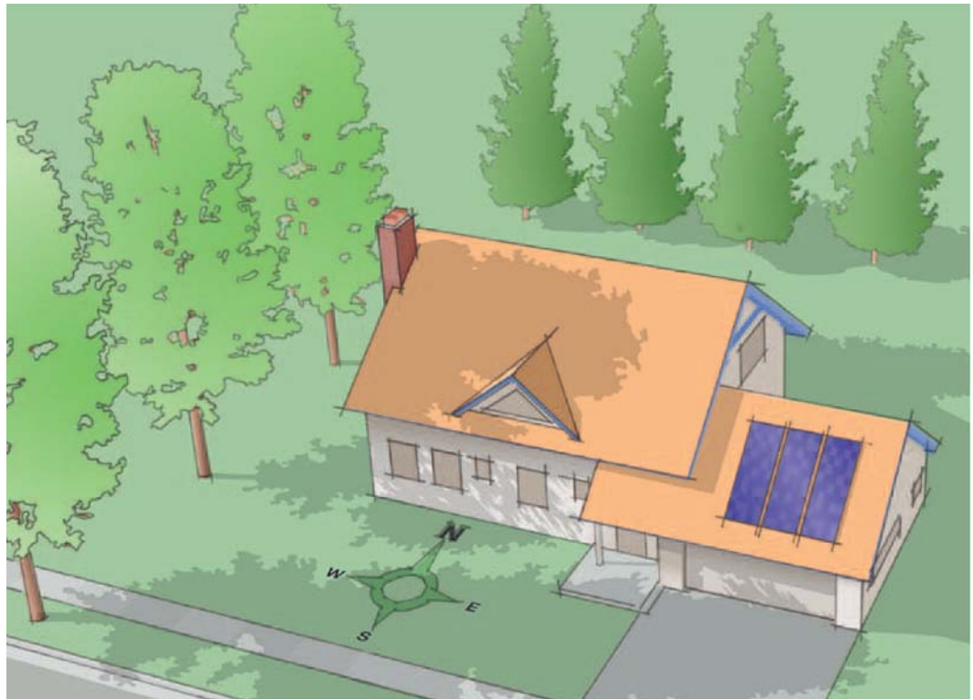
Figure 6-3 – The proposed layout for the system should be verified by the installer to ensure that the collectors are oriented properly and that shading will not be a significant issue.
