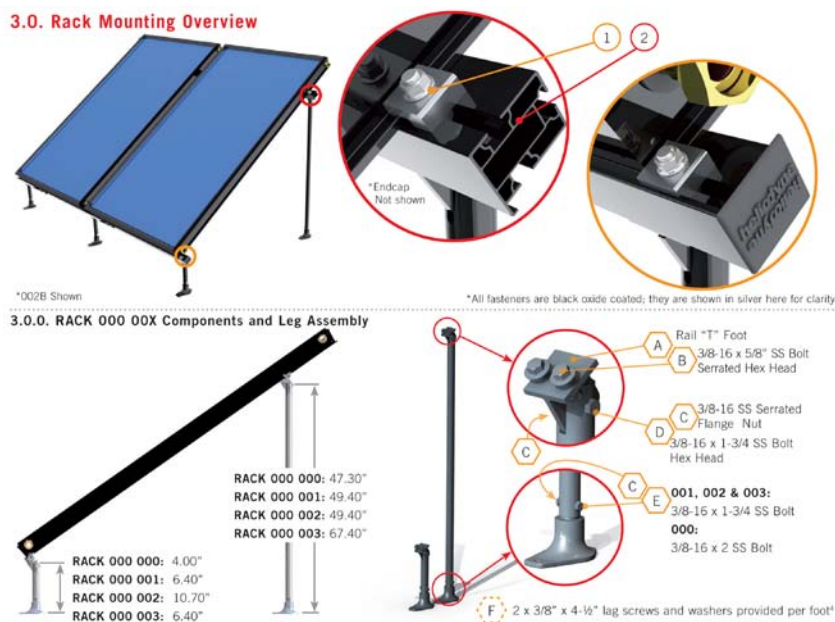
Figure 8-5 — Proprietary flat plate collector mounting rack. (Courtesy of Heliodyne)
