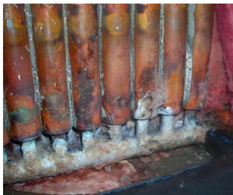
Figure 10-26 – Corrosion in a copper tube heat exchanger.
