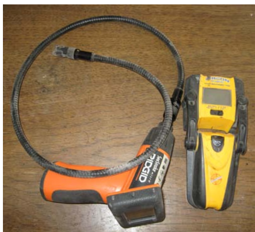
Figure 7-2 — A camera-type boroscope and a higher-end stud finder can help with installation planning.
