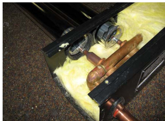
Figure 10-15 — Cutaway view of an evacuated tube collector manifold. The tube on the right is fully inserted into the dry socket of the manifold. The condenser bulb of the heat pipe on the left is visible prior to insertion into the dry socket.
