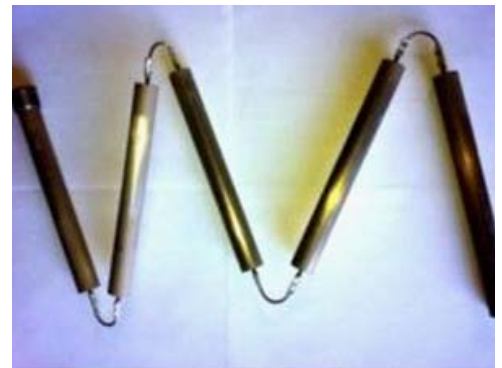
Figure 10-10 — Chain-style anodes can be used for locations where there is not sufficient clearance to replace an anode rod.
