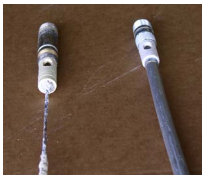
Figure 10-8 — The anode rod on the left will no longer protect the tank from corrosion and must be replaced by a new anode rod (right).
