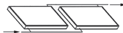
Figure 8-23 — Plumbing harp-style flat plate collectors in parallel when oriented landscape requires extra external piping. (Courtesy of NYSERDA)
