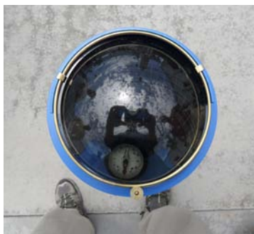
Figure 6-9 – Solar Pathfinder shade analysis tool.
