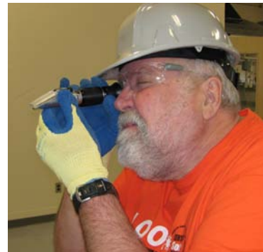
Figure 8-52 — Checking propylene glycol concentration using a refractometer.
