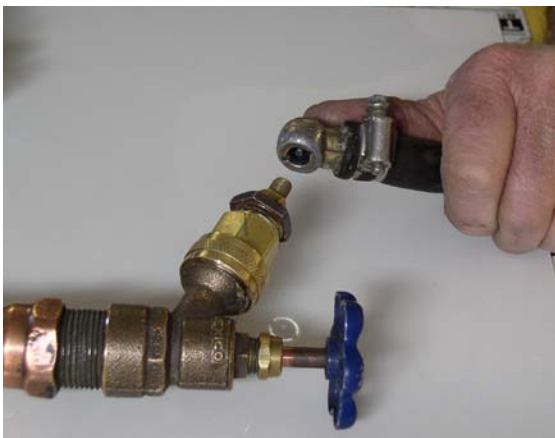
Figure 8-37 – Filling the system with compressed air.
